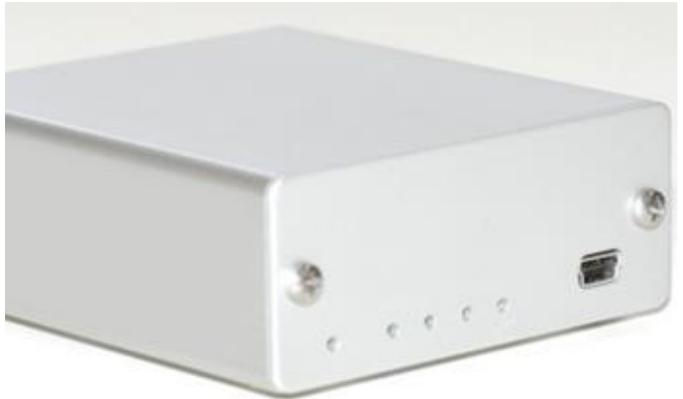
The opto-electronic interface receives optical signals from the handheld devices in the MR suite, and converts them into electronic signals for the computer.
