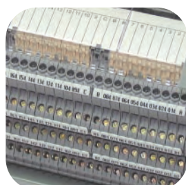
The T/Guard2™ comes with industrial-grade relays featuring galvanic isolation
